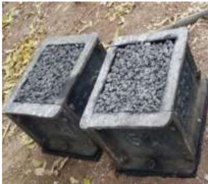
Fig. 3 Moulding of Concrete
