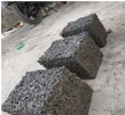
Fig. 4 Demoulding of Concrete
