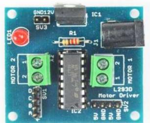
L293D may be a typical Motor driver or Motor Driver IC which allows DC motor to drive on either direction. L293D may be a 16-pin IC which may control a group of two DC motors simultaneously in any direction. It means you'll control two DC motor with one L293D IC.
