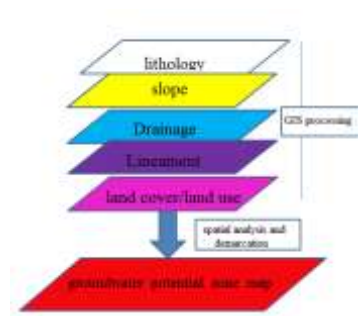
Fig -1: GIS technology used in spatial integration and analysis to demarcate basin groundwater recharge potential zone
