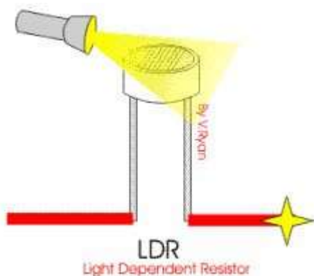
Fig-8. Working Principle of LDR
