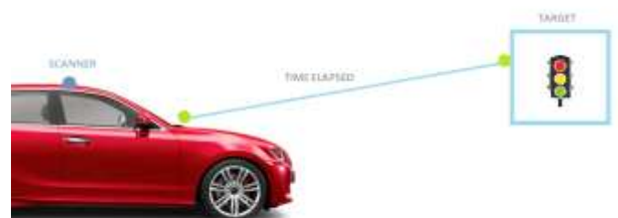
Figure 7: Simple representation of LIDAR used in cars
