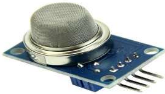
Fig -7: Gas sensor
