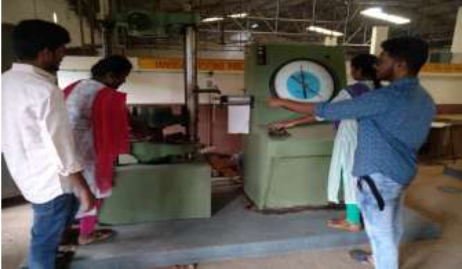
Fig -1: Compressive Strength Test on Bricks
