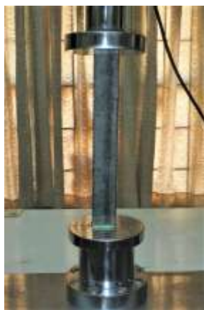
Fig 19: Compression testing of 1% CNT infused GFRP Beam
