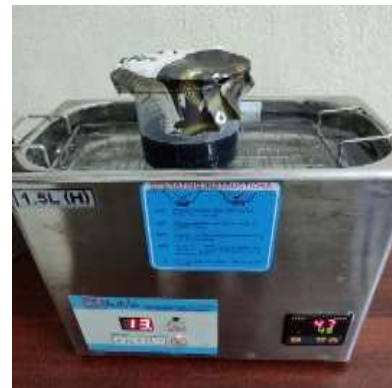
Fig 2: Ultrasonication of Resin CNT mixture
