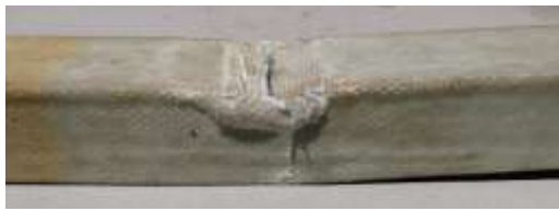
Fig 12: Plain GFRP box beams after failure
