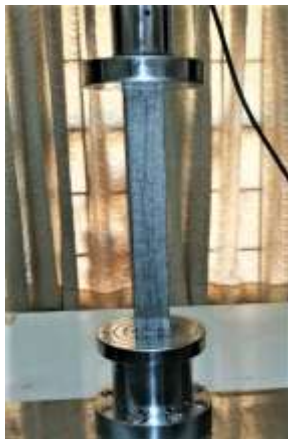
Fig 17: Compression test on 0.5% CNT infused GFRP Beam
