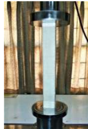
Fig 15: Compression test on plain GFRP Beam
