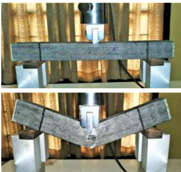
Fig 9: Bending Test for 1% CNT Infused GFRP Beam
