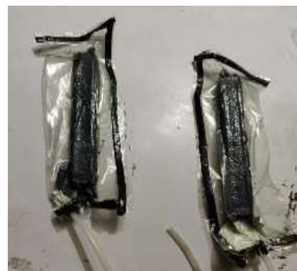
Fig 3: Vacuum Bagging of GFRP Box Beams
