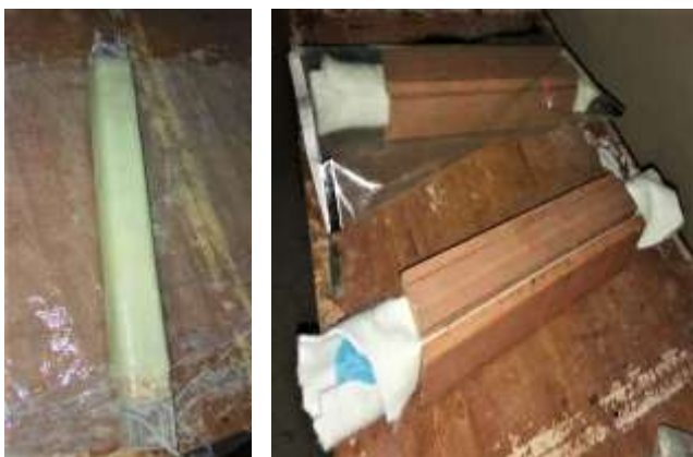
Fig 1: Fabrication of GFRP Box Beams using Hand lay-up
