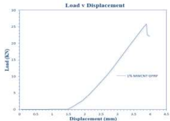
Fig 20: Load vs Displacement graph for 1% CNT infused GFRP Beam
