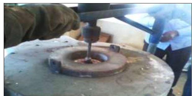
Fig -2: Stir Casting of Al/TiC MMC
