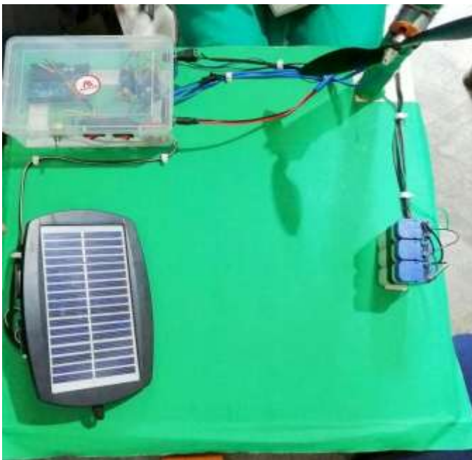
Fig.4.2. Hardware Implementation of Renewable Energy Based Interleaved Boost Converter for the Application of BLDC Motor
