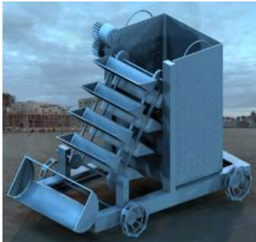
Fig. 5 Working Model of Sewage Cleaning Machine
