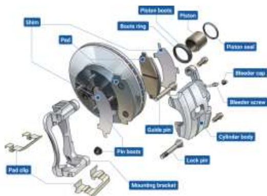
Fig – 13: Disc brake components of automobiles
