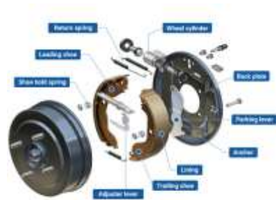
Fig – 5: Drum brake components
