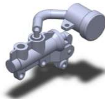
Fig - 18: Design of master cylinder
