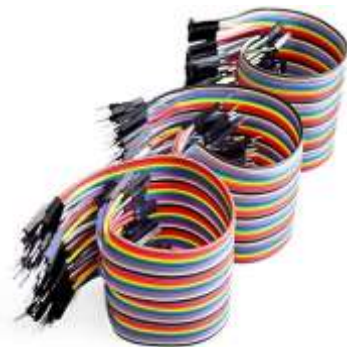
Fig-5: Jumper Wires
