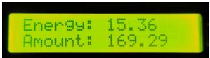
Fig 9: Meter readings after switching ON the load
