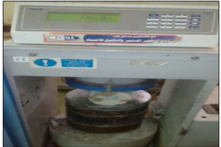
Fig- 5: cylinder (100 mm *200 mm) during splitting strength test
