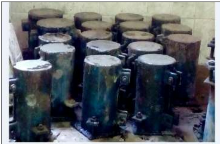
Fig- 2.a: Cylinders (100 mm *200 mm) during casting
