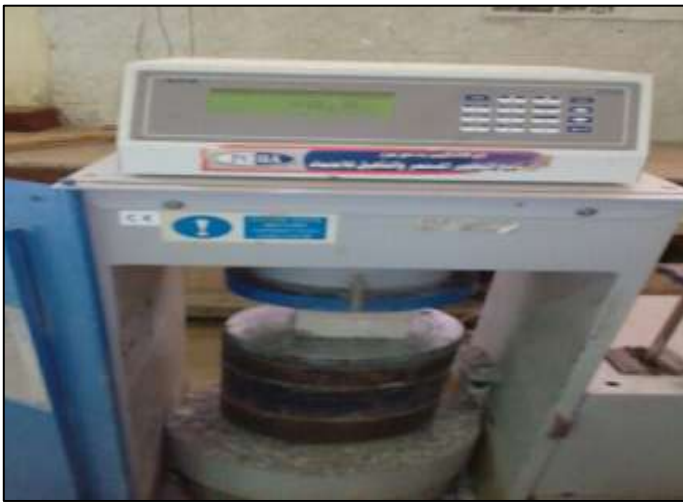
Fig- 4: Cube (100 mm *100 mm*100mm) during compressive strength test
