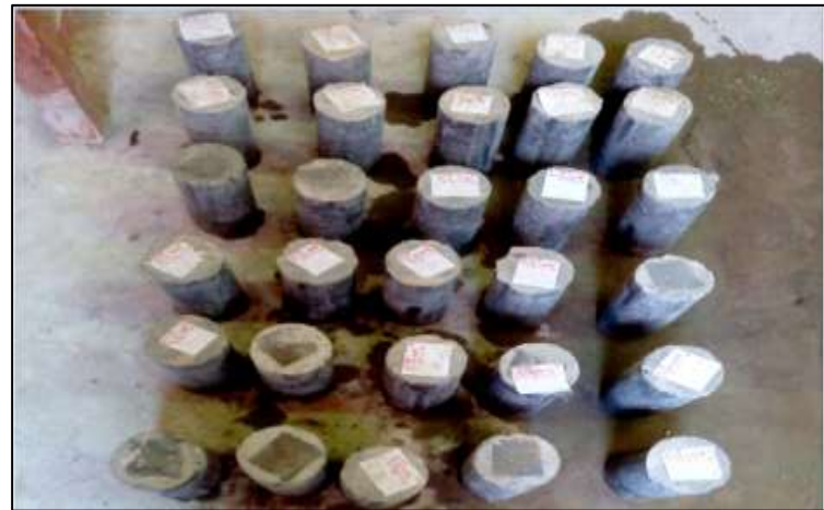
Fig- 2.b: Cylinders (100 mm *200 mm) after hardening
