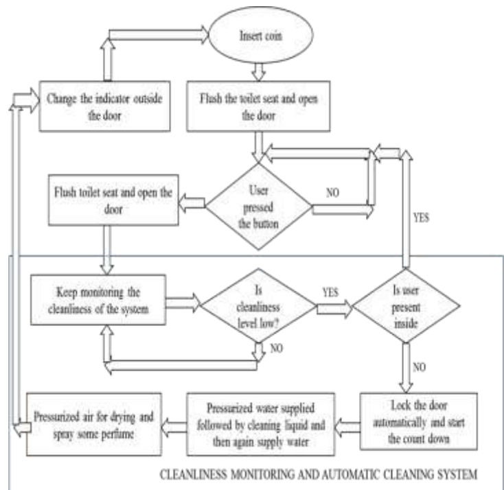
Figure 6.3 Flow diagram of overall system
