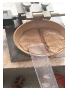
Fig -2: Liquid limit
