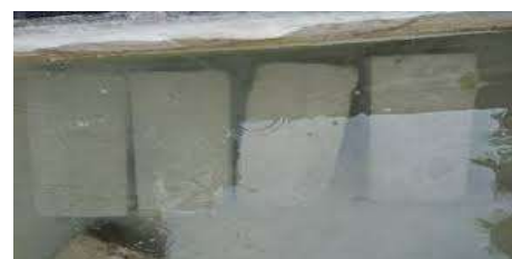
Fig.7. Water absorption test
