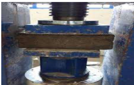
Fig.6. Compressive strength test
