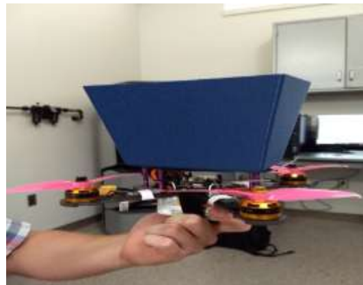
Fig 1: fully assembled quadcopter with payload basket.
