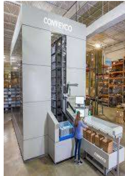
Fig - 7: VLM type Storage System with Security Features
