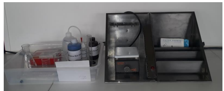
Figure-5 Apparatus of methylene blue test (MBT).
