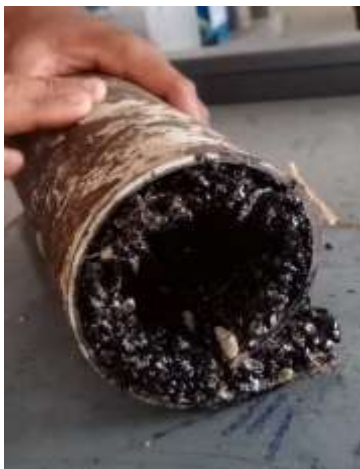
Fig -3: Rolled prefabricated wearing course
