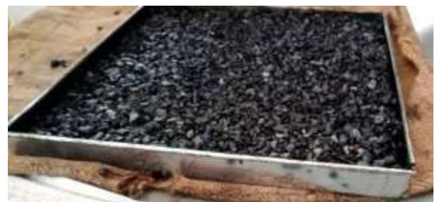
Fig -1: Precast of the bituminous unit
