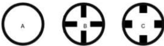
Fig- 2 (b) Cross section of absorber tube A) plain tube, B) rectangular heat transfer enhancer, C) square heat transfer enhancer
