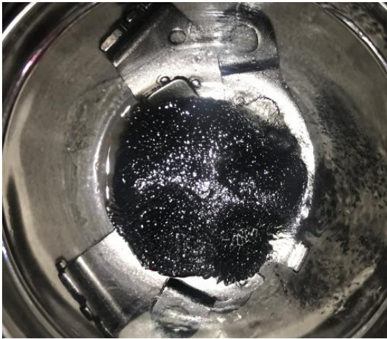
FIG. 3: THE MANUFACTURED MAGNETO-RHEOLOGICAL FLUID
