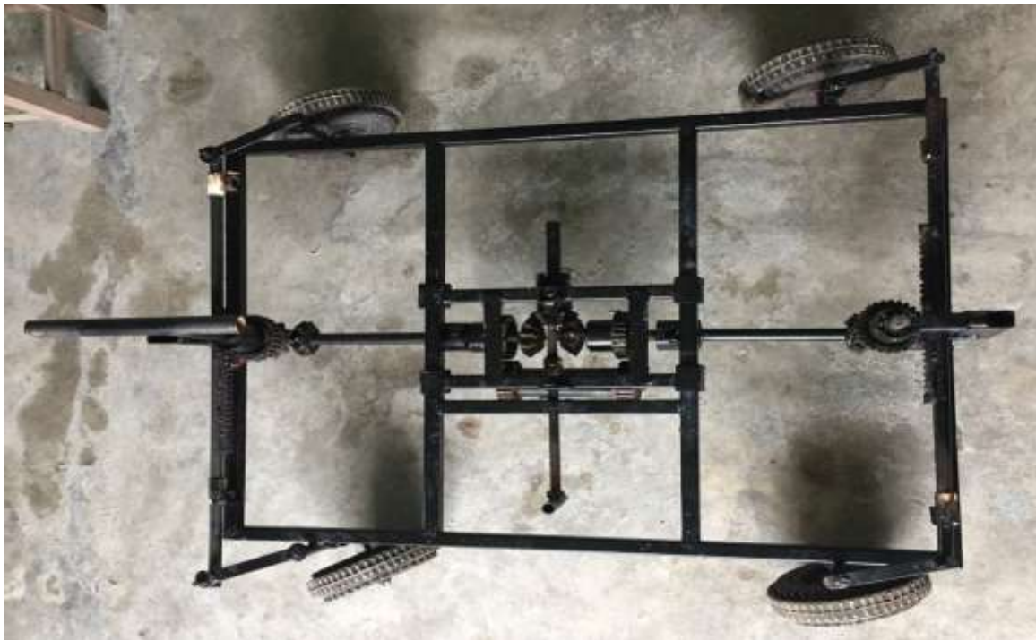
Fig 6: Top view of the IN-PHASE steering mechanism
