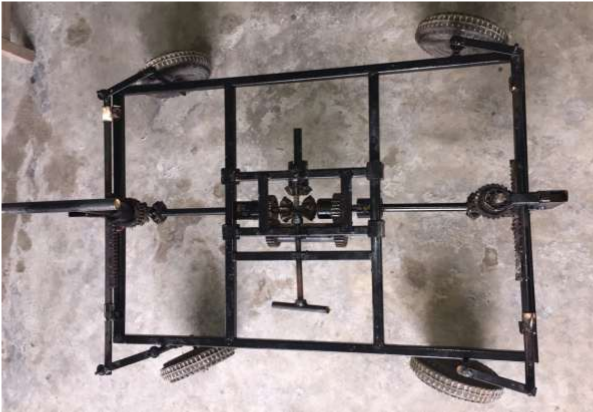
Fig 4: Top view of the COUNTER-PHASE steering mechanism
