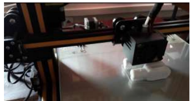
Fig -9: fabrication of fork ends
