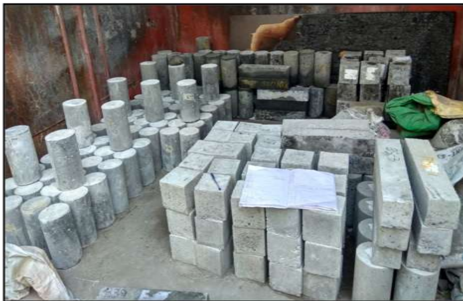
Fig 4. Casted specimens of Cubes, Cylinders and Prisms
