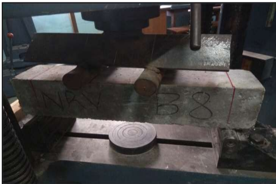
Fig 10. Specimen subjected to flexural strength
