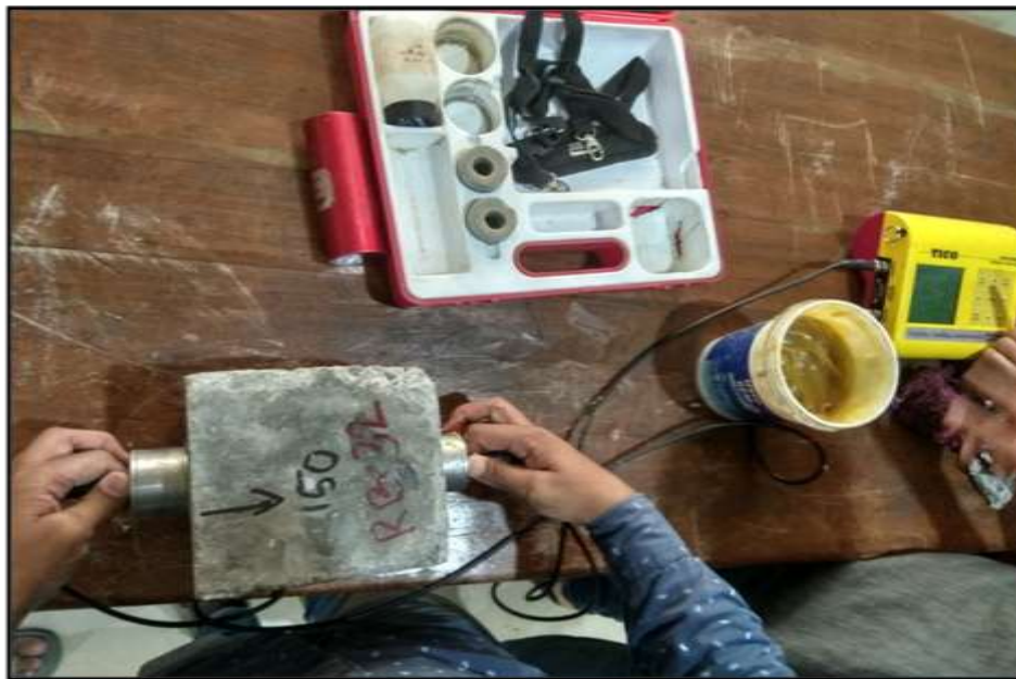
Fig 7. Ultrasonic Pulse Velocity Test of Cube
