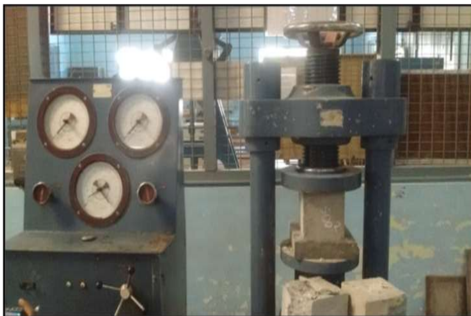
Fig 8. Specimen subjected to compressive strength
