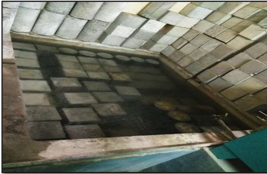
Fig 5. Curing of Specimens
