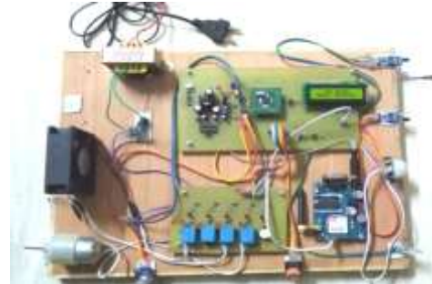
Fig 7:- Photograph of fabricated project Smart Industrial Control and Safety System
