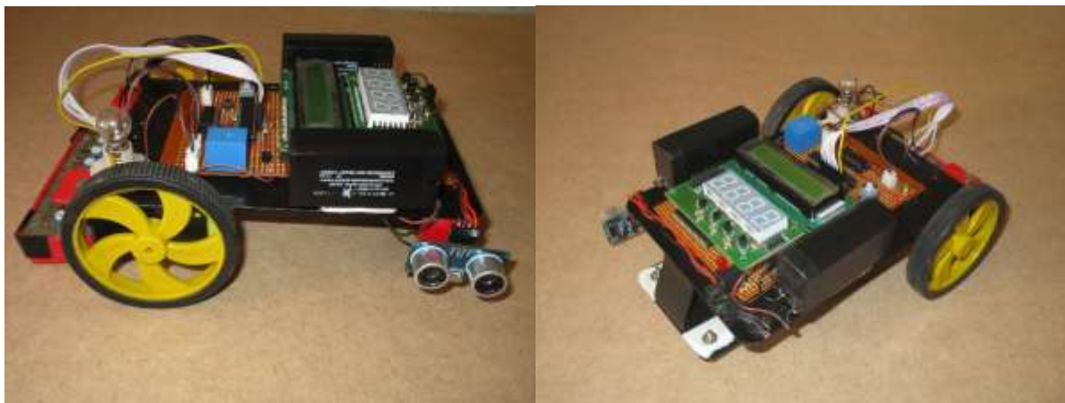
Fig 2: Implemented Line follower prototype model
