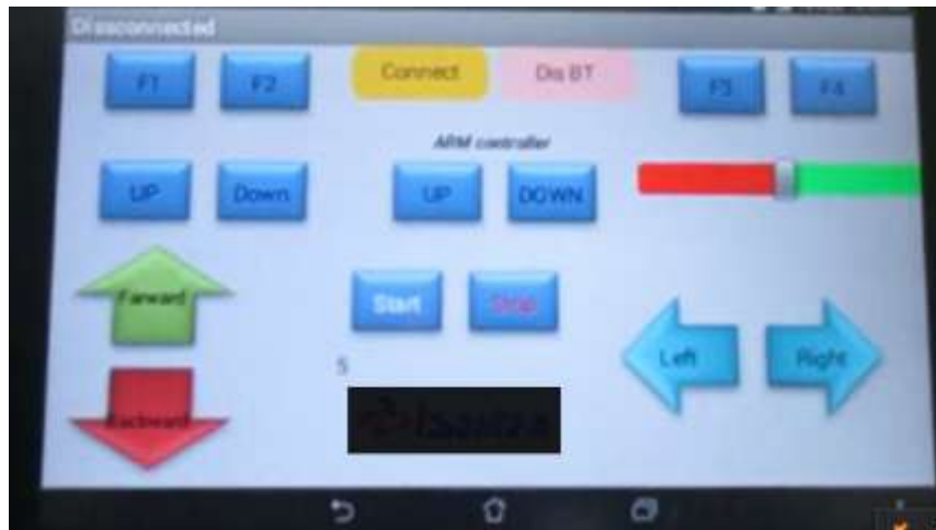
Fig 3: Bluetooth control panel for pick and place robot
