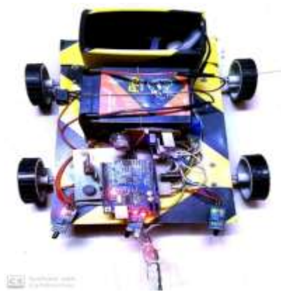
Fig.9 Hardware of fire fighting robot
