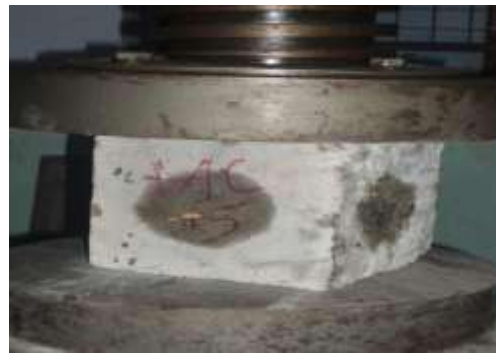
Fig -4: Compressive Strength Testing Arrangement
