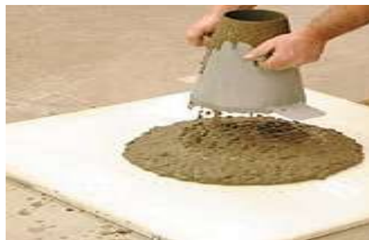
Fig- 3: Slump test
