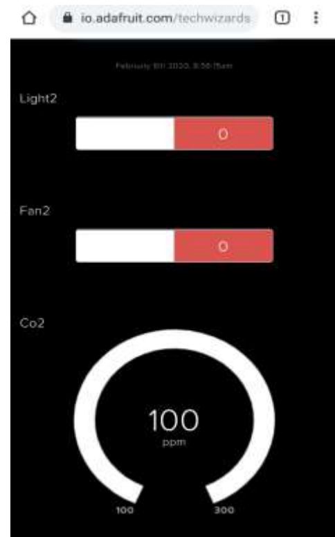
Fig -7: Value of Co2 gas displayed in Adafruit dashboard.
