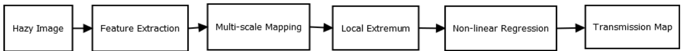
Fig. 5 The architecture of DehazeNet. DehazeNet conceptually consists of four sequential operations (feature extraction, multi-scale mapping, local extremum and non-linear regression).
