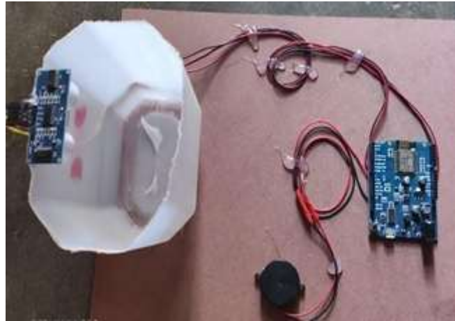
Fig 2.IOT based fuel monitoring system
