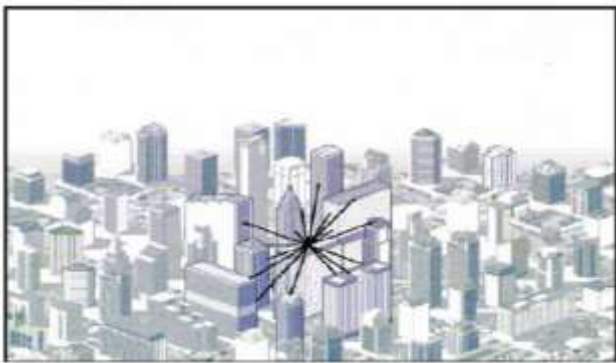
Fig.1.7 point to multipoint architecture
