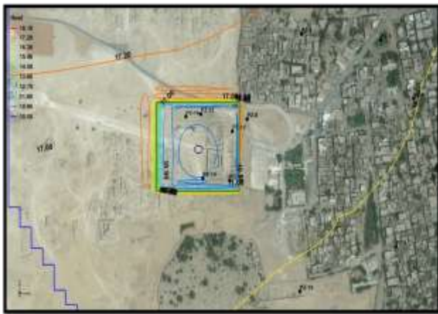
Barrier with vertical well pumping 400 m 3 /d
