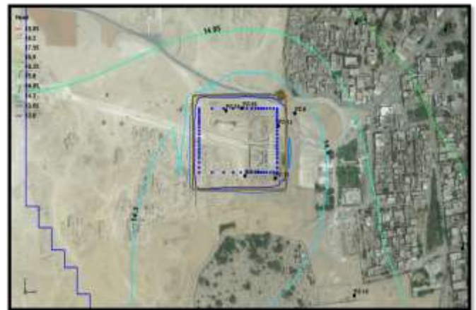
Figure (2) Calculated Groundwater Levels for Liner Drain with barrier
