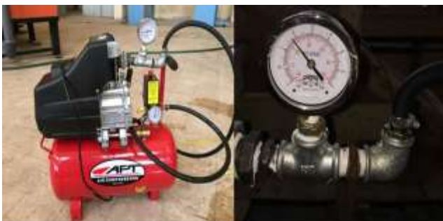
Fig .5: Air compressor to compressed air to 2 bars in backwash process
