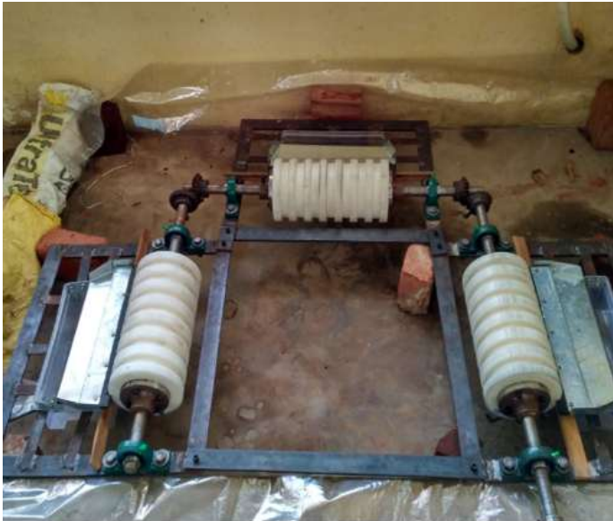
Fig3: Final Fabricated setup of the skimmer
