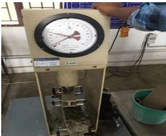
Figure 9.1: Flexural strength test setup
