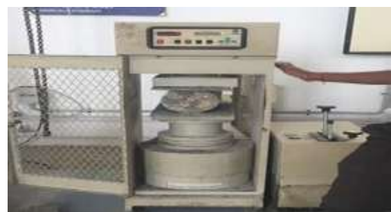
Fig 8.1 Cylinder mounted for Split tensile
