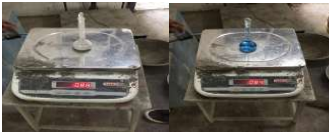
Figure 3.1 Specific Gravity Test on Cement
