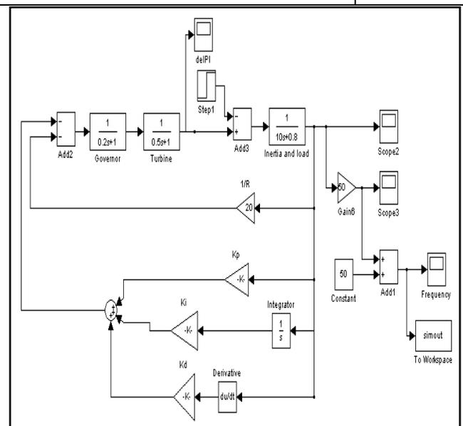
Fig. 2: Simulink Model of Isolated power system
