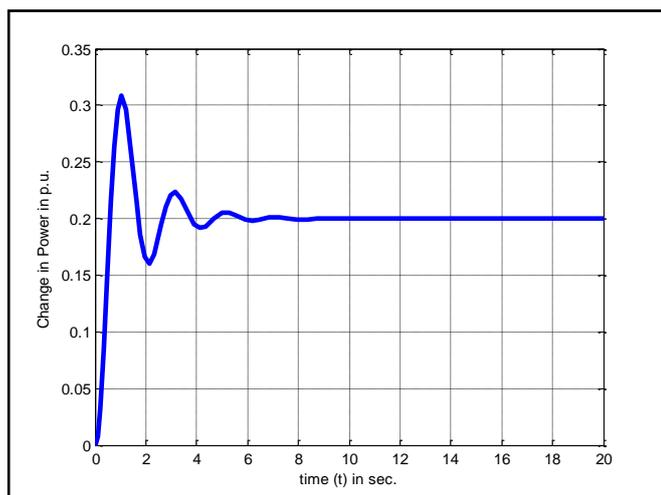
Fig. 10: Mechanical Power output by Turbine with Tuned PID by ZN Method
