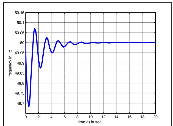
Fig. 6: PID with  $K_p = 50, K_i = 30$  &  $K_d = 10$
