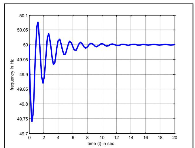
Fig. 7: PID with  $K_p = 80, K_i = 40$  &  $K_d = 15$
