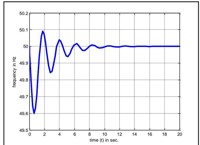
Fig. 5: PID with  $K_p = 30, K_i = 20$  &  $K_d = 5$
