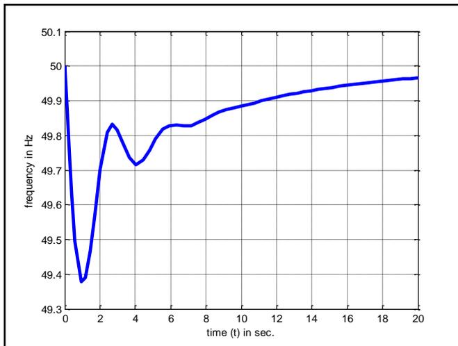
Fig. 3: PID with  $K_p = 5, K_i = 3$  &  $K_d = 1$
