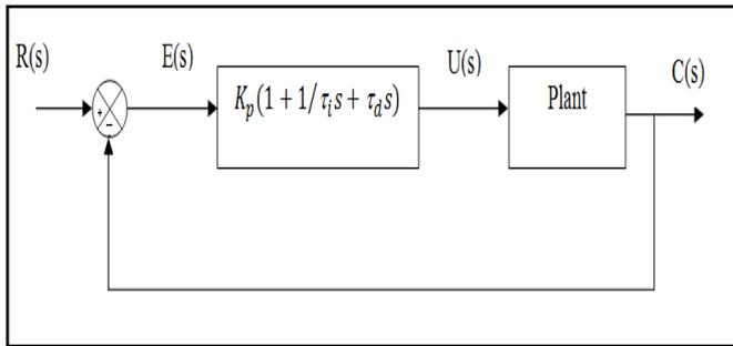
Fig.1: PID Control Configuration
