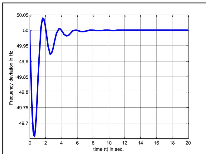
Fig. 9: Frequency Deviation with Tuned PID by ZN Method
