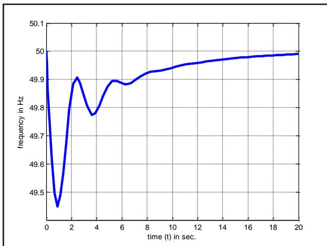
Fig. 4: PID with  $K_p = 10, K_i = 5$  &  $K_d = 2$
