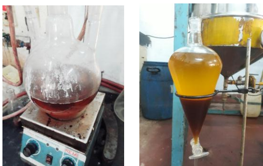
Fig: 2.3. (a) Magnetic Stirrer Apparatus (b) CSME + Glycerol Separation
