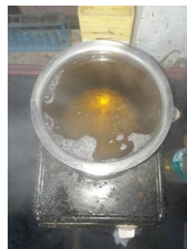
Fig: 2.4. Heating of CSME after washing to remove excess water vapor
