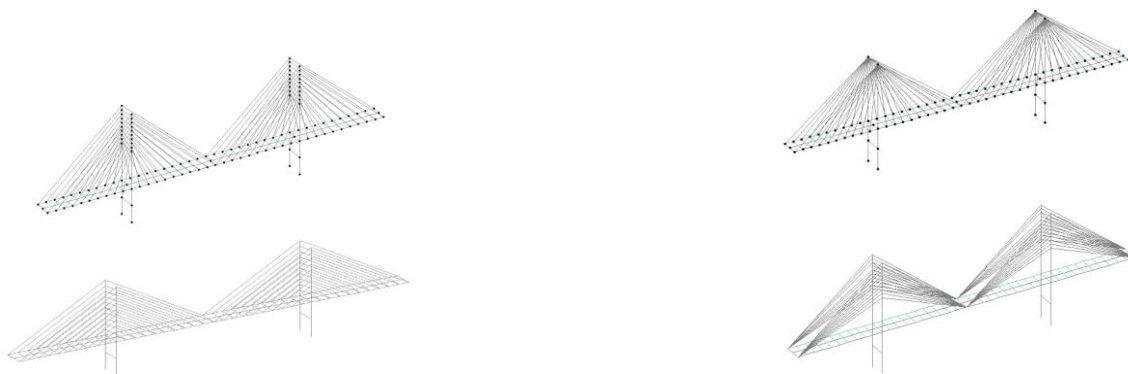
Fig. 1: H shape tower with different cable arrangement
