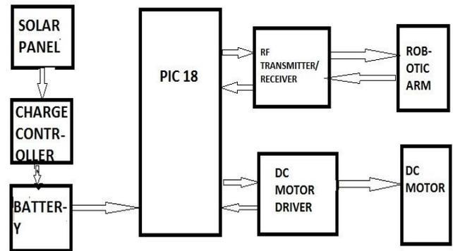
Fig -3: Block Diagram of the Robot
