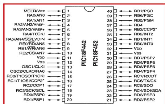
Fig -1: Pin Diagram of PIC 18
