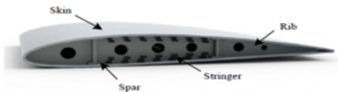
Fig - 3: The typical Airframe structure Lifting
