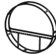
Fig - 11: The meshed model of Fuselage cross/Floor beam
