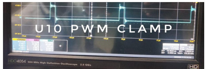
Figure 11 Vgs of aux/clamp MOSFET.
