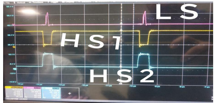
Figure 10 Vgs of Primary Main MOSFET (pink), Secondary Forward MOSFET (blue), Freewheeling MOSFET (yellow).
