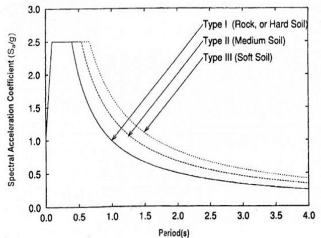
Fig. 3.1 Response Spectra for Rock and Soil sites for 5% Damping
