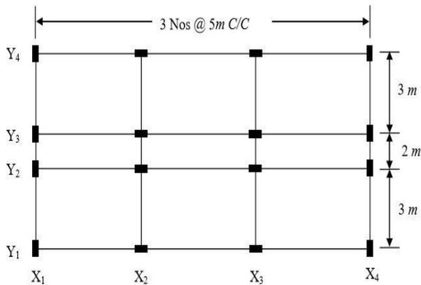
Fig. 4.1 Plan of the RC Framed building
