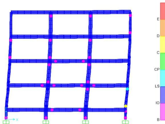
Fig 5.2 Deformed Shape and Hinge Formation after Pushover Analysis
