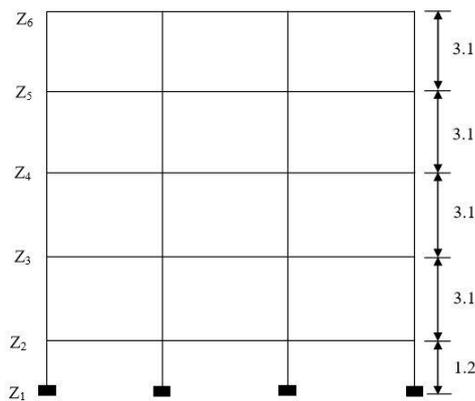
Fig. 4.2 Elevation of the RC Framed Building
