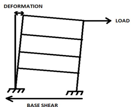
Fig. 1.1 Pushover Mechanism
