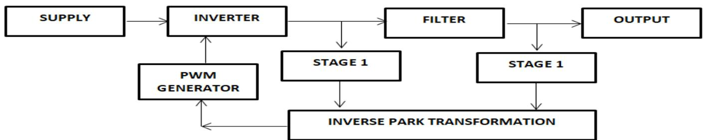
Fig -1: Flow model of inverter design
