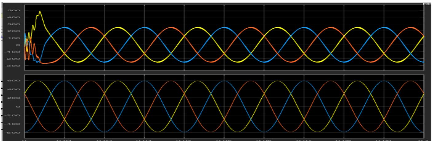
Fig -3: Current and Voltage waveform of three phase feedback SPWM inverter
