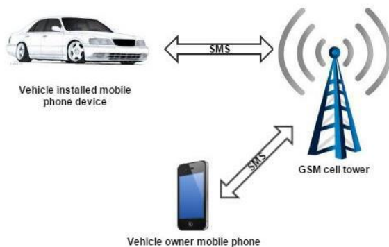
Fig.3.2. Physical architecture of the theft alert function
