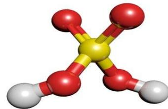
**Fig -2.3** Structure of H<sub>2</sub>SO<sub>4</sub>
