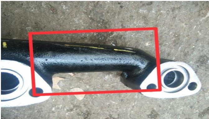
Fig -7: Cold Shut Defect
