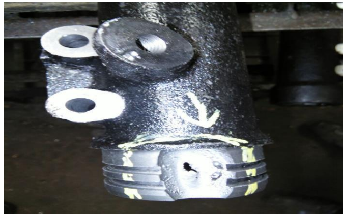
Fig -13: Gas Porosity Defect
