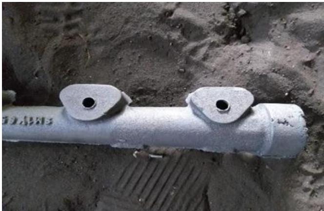
Fig -10: Sand Inclusion Defect
